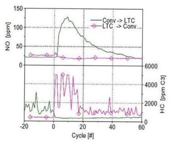
Figure 7: Non-transient mixed mode switches between LTC and conventional diesel combustion [30]
