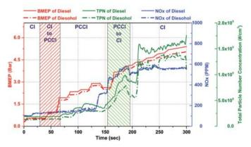
Figure 6: Variations in NOx and TPN emissions with BMEP during different combustion modes and mode transitions [27]
