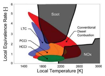
Figure 2: Local equivalence ratio-flame temperature correlation of different low temperature combustion techniques for simultaneous control of soot and NOx formation [1]
