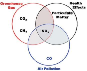
Figure 1: Engine exhaust emissions and associated health and environmental effects
