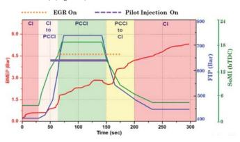
Figure 5: Fuel injection parameters and EGR for CI and PCCI combustion mode switching
